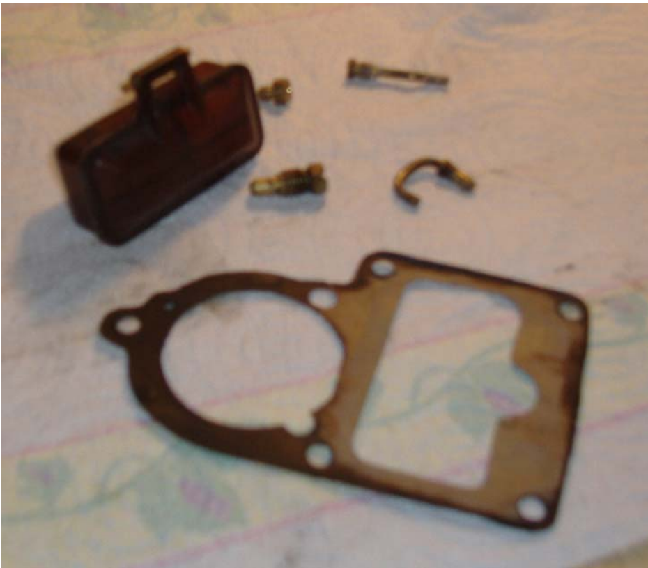
Figure 5 – Float and Jet Parts Pristine, Gasket Cracked at Screw Hole (Nearest Idle Jet).
