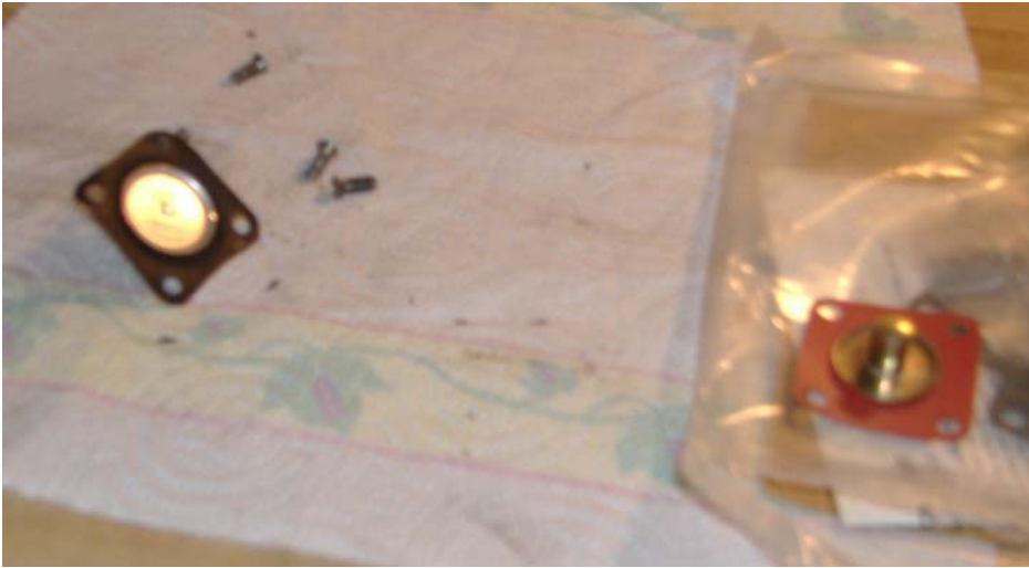
Figure 6 – Old Accelerator Pump Diaphragm is the Black Neoprene Part on the Left, Still Quite Pliable. The Metal Clinch Disks Were Loose, Causing the Leak. The New Red Neoprene Part is on the Right.
