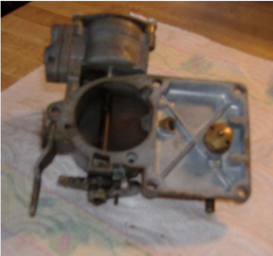
Figure 3 – View Into Top Cover: Note Pristine Float Valve and Clean Casting.
