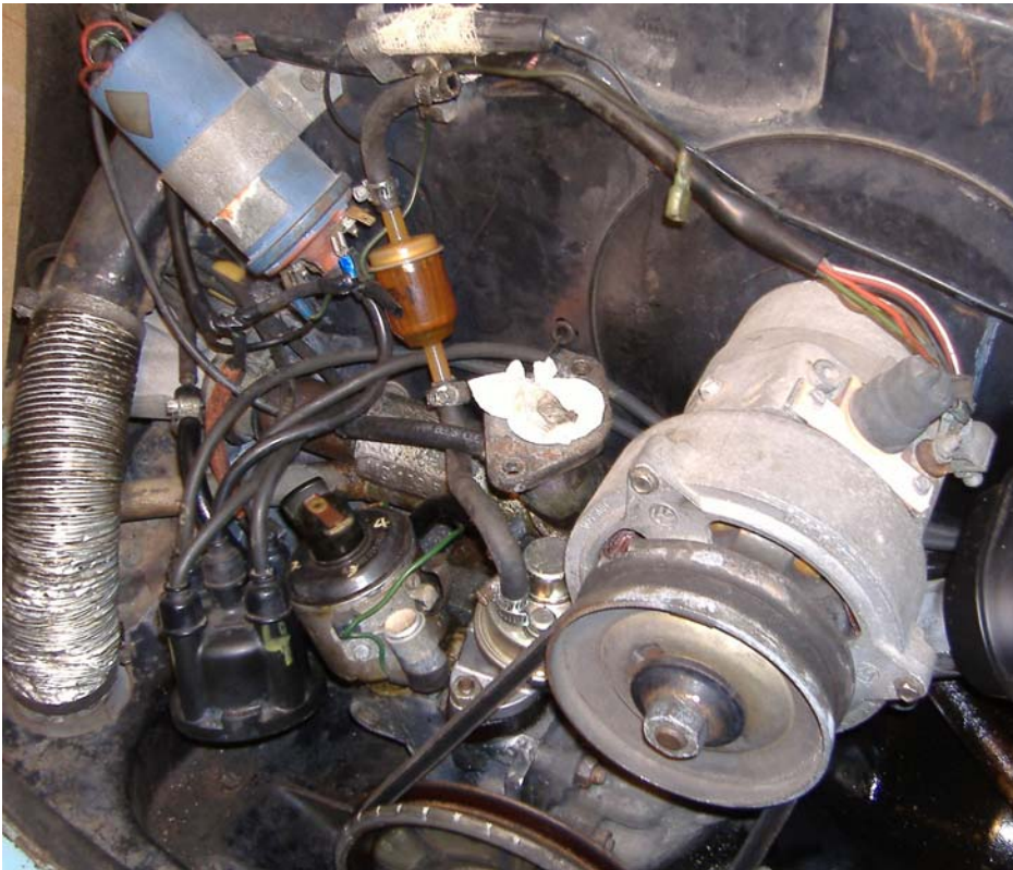
Figure 7 – View of the Engine with Carburetor Removed. Note the Pristine Fuel Filter, and the Excellent Condition of Black Neoprene Fuel Lines.
