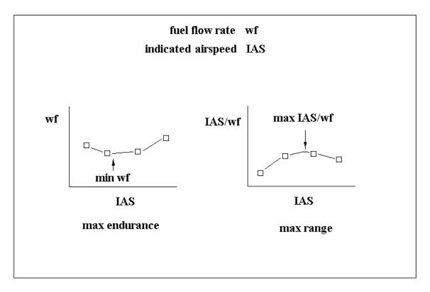
A very simple procedure can determine flight speed for best endurance (time aloft) and for best range (not the same flight speed as best endurance). A real flight test enterprise would reduce everything to standard conditions and normalize it, but most light plane pilots need not go to such trouble. You can do this if you have a fuel flow rate meter, which most experimental aircraft have. This will even work in turbine aircraft.
