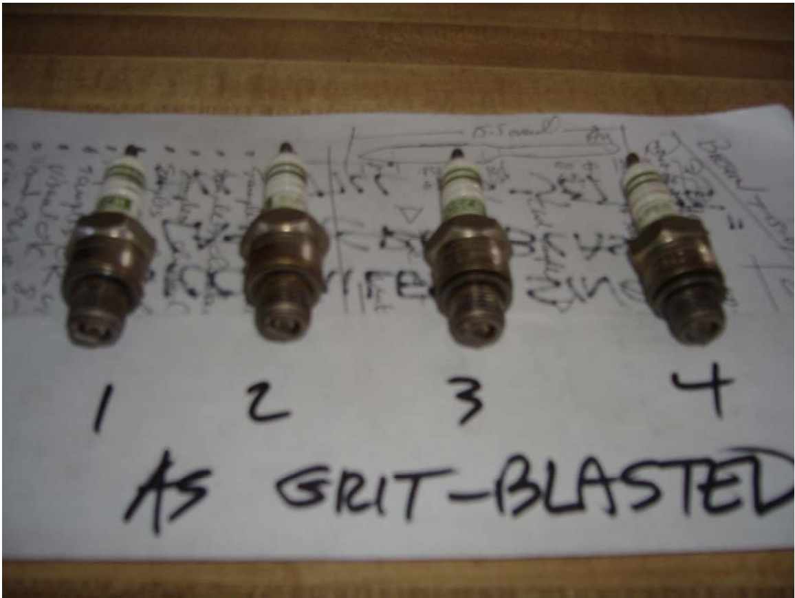
Figure 3. – Plugs Ready-to-Install Look Exactly as They Appeared Freshly Removed
