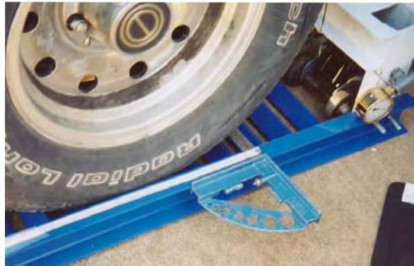
Figure 10 – Locate tire position on scale: measure both sides of tire and average the positions
