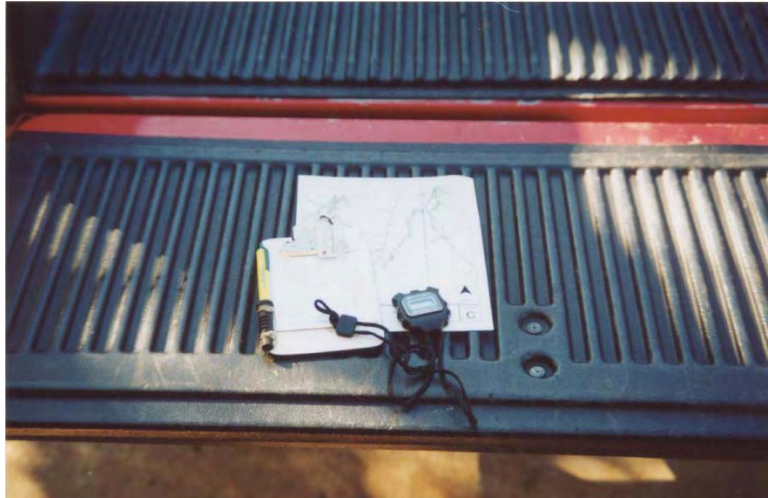
Figure 16 – On-board test tools for a coastdown test run
