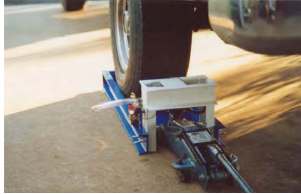
Figure 9 – Prybar scale in actual use: prybar is the blue structure, hydraulics are in white lift bridge
