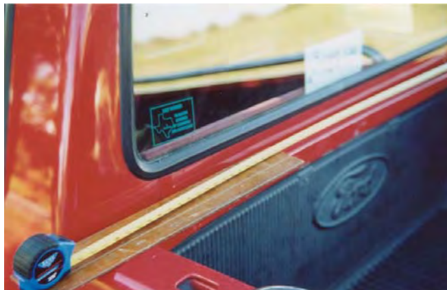
Figure 11 – Measuring across the vehicle as part of determining frontal area
