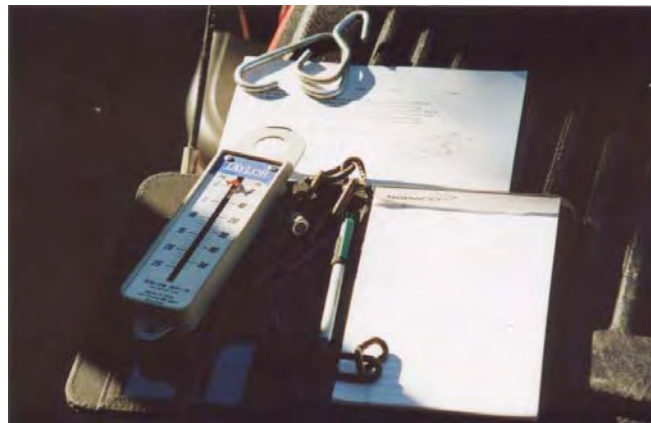
Figure 15 – Tools for driveway pulls are very simple
