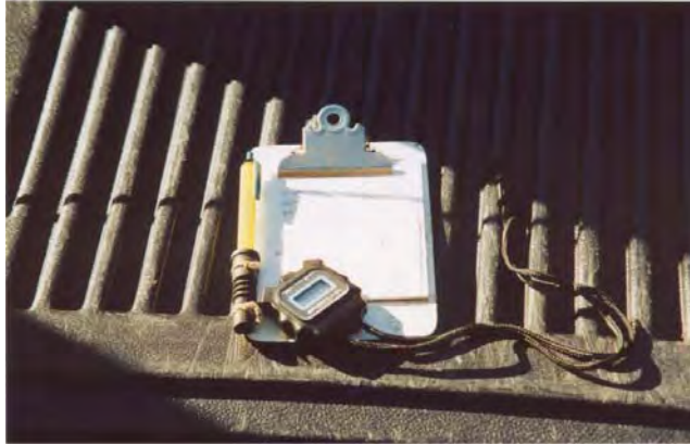
Figure 4 = Tools required to calibrate a speedometer (delete stopwatch for odometer)
