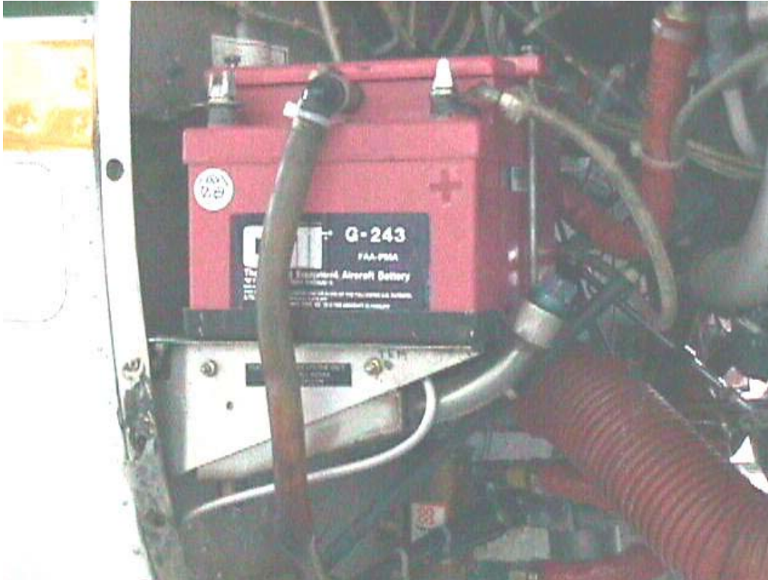
Figure 5 – Firewall-Mounted Start Canister in Cessna 152 Engine Compartment
